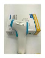
Infrared pyrometer for measuring surface temperature in the range from -30 to +5000C.
